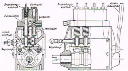
The four-cylinder Bosch plunger pump of 1923
