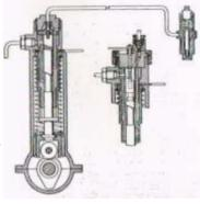
that an upper scroll face machined on it could control the suction port and a lower helix could take care of the return to the suction side (see illustration) was developed.
