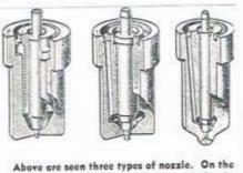
Above are seen three types of nozzle. On the left is the Acro-Lang two-part pintle, in the centre is the Bosch single-piece and on the right the Bosch multi-hole type
